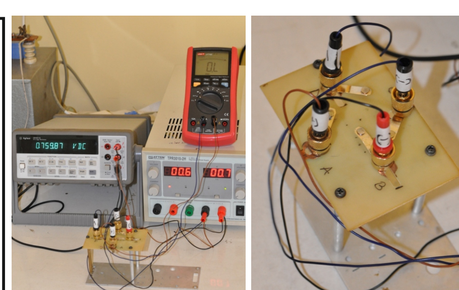
Fig. 2. Experimental setup for the measurement of sheet resistance of AgNWs on PMMA/PET transparent conductig films
