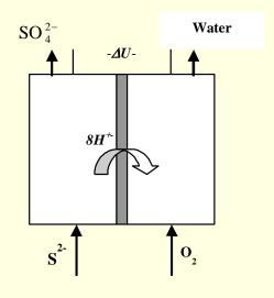
Anode:  $S_2^- + 6OH^- - 6e^- = SO_3^{2-} + 3H_2O$ ,  $E_0^- = -0.61 \text{ V}$
